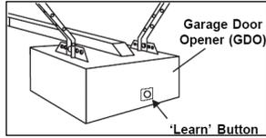
B) Next press the TEST SWITCH button on the front of Protectrix™. You may need to press TEST SWITCH two to three additional times. The garage light likely will turn off or blink and the learn light near the learn button should flash or go off also. Protectrix will beep and blink. Protectrix is now programmed and can open and close your garage door.
